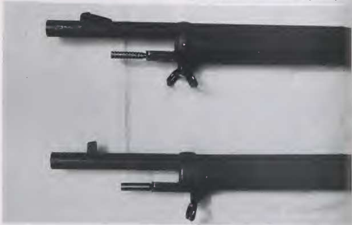
Figure 16 The distinctive nose cap feature which makes the W.A. issue Martini-Enfield rifles unique. These rifles are the only Australian Martini-Enfield rifles which fix the Pattern 1888 sword bayonet. The upper rifle is the Martini-Metford Mark I, W.A. Pattern, the first W.A. service rifle to fix the Pattern 1888, the lower is the Martini-Enfield Mark I, W.A. Pattern. (Photo R. Sinclair).
